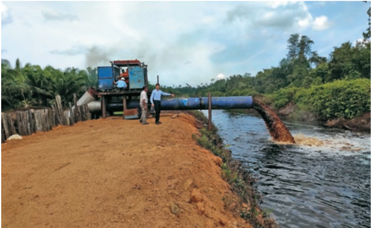
A large water pump to help mitigate periodic flooding at Runtu Estate, Kalimantan.
