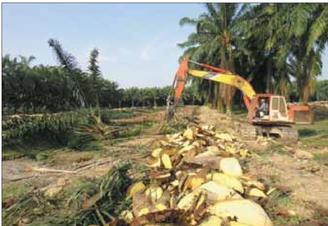
*Excavator chipping the trunks of the old stand in support of our 'zero-burn' policy. The chips are recycled as mulch which adds organic matter and retains moisture.*
