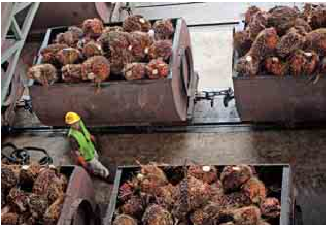
Loaded FFB cages ready for sterilization.
