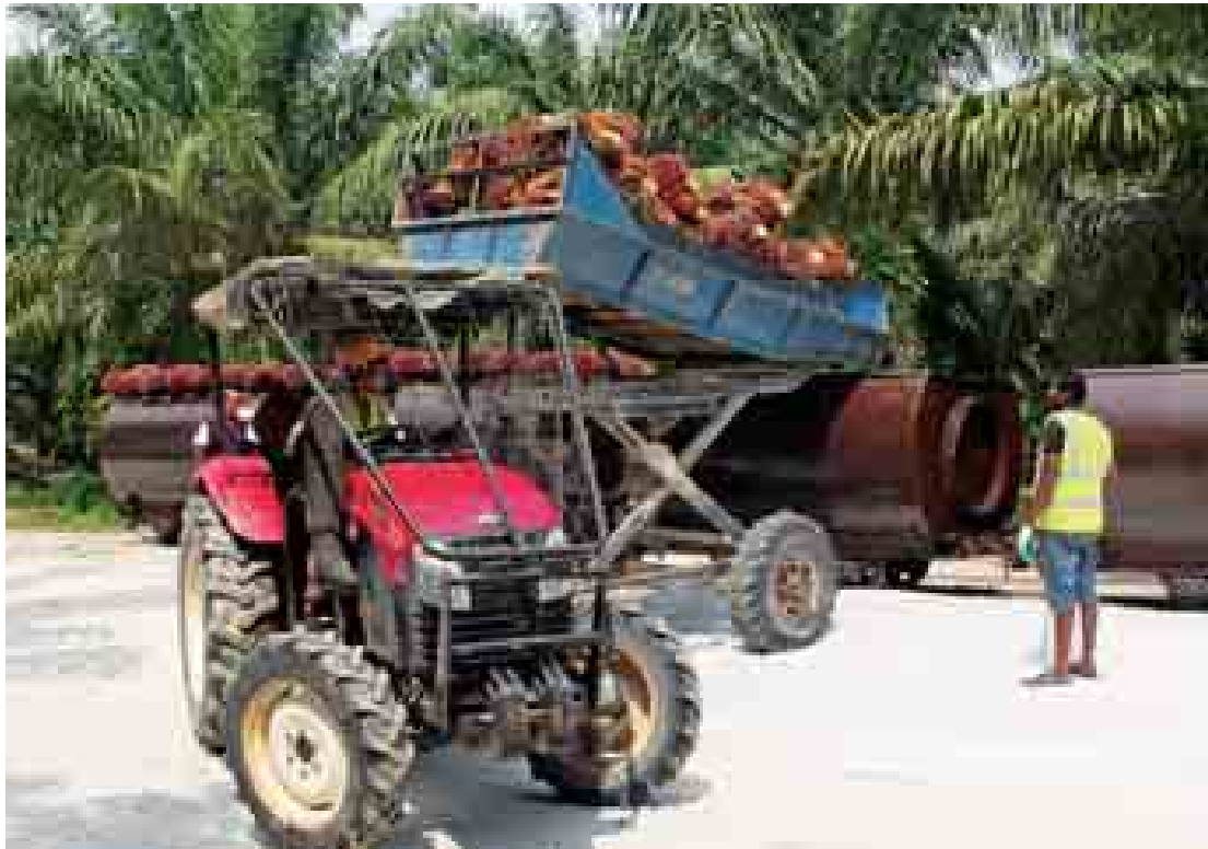
Loading of evacuated bunches from the fields into the 2MT cages using scissor lift trailer.
