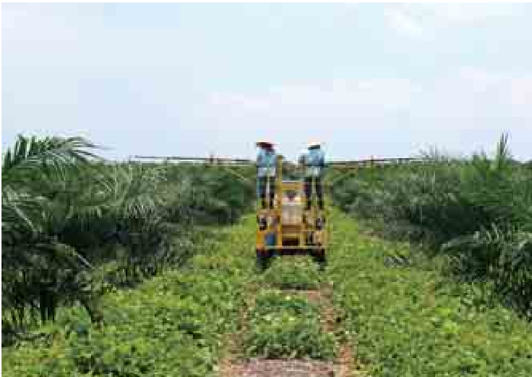
Mechanised spear drenching for oryctes beetle control in immature oil palms.
