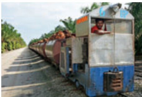
Front Cover: UP's unique light Railway System stretching over 530 km's in length ensuring an efficient transport of harvested fresh fruit bunches to the palm oil mill.
