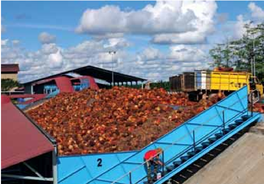
The Lada Mill FFB ramp which can hold upto 700MT of FFB at any one time.
