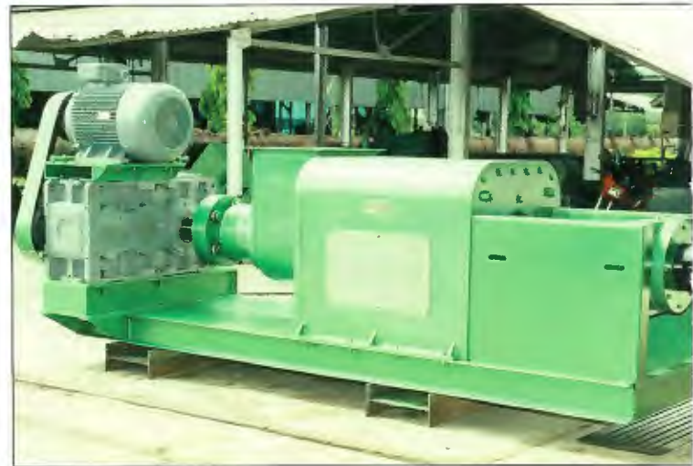
United Plantations Berhad's designed Empty Bunch Press, which was developed after several years of experimentation, has produced excellent results in as much as it has increased the extraction rate of Palm Oil by 0.2%. It has, at the same time, reduced the moisture content of the empty fruit bunches by about 30%.
