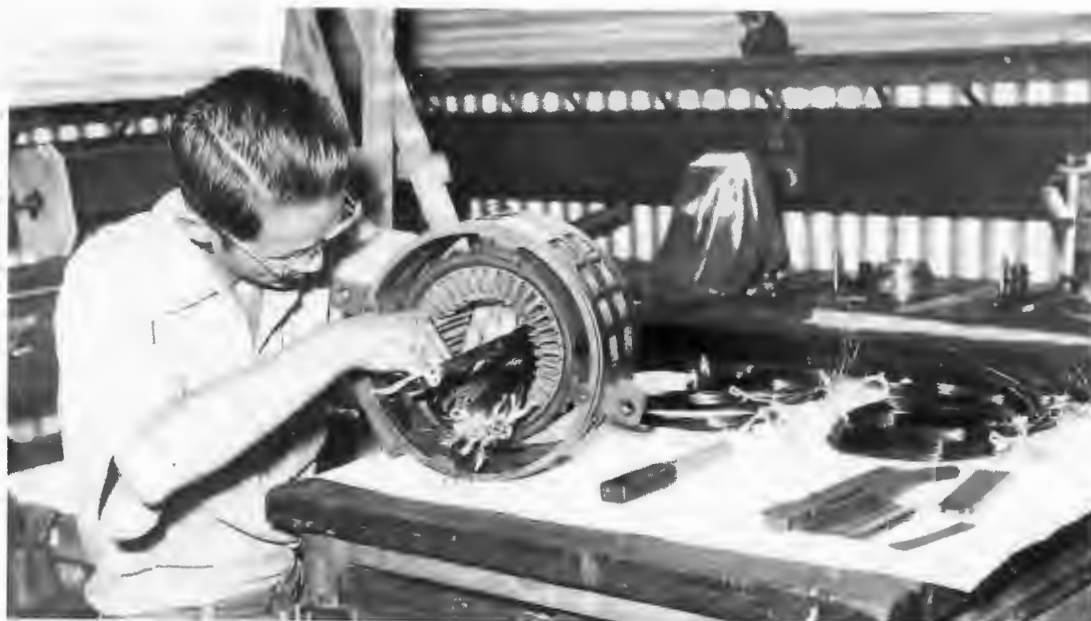
Rewinding of electrical motors at Ulu Bernam Engineering Department in the late 1960's.
