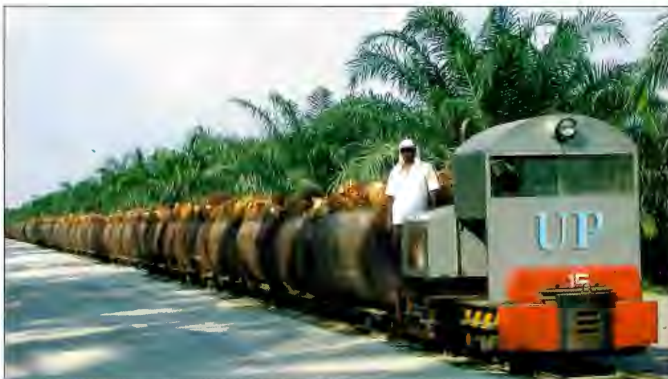
A part of UP's unique 500km long light rail system of transporting fresh fruit bunches to the mill in 2006.
