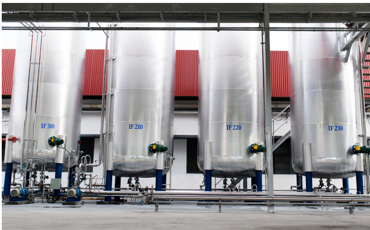
Stainless steel tanks for the storage of high quality products at Unitata.
