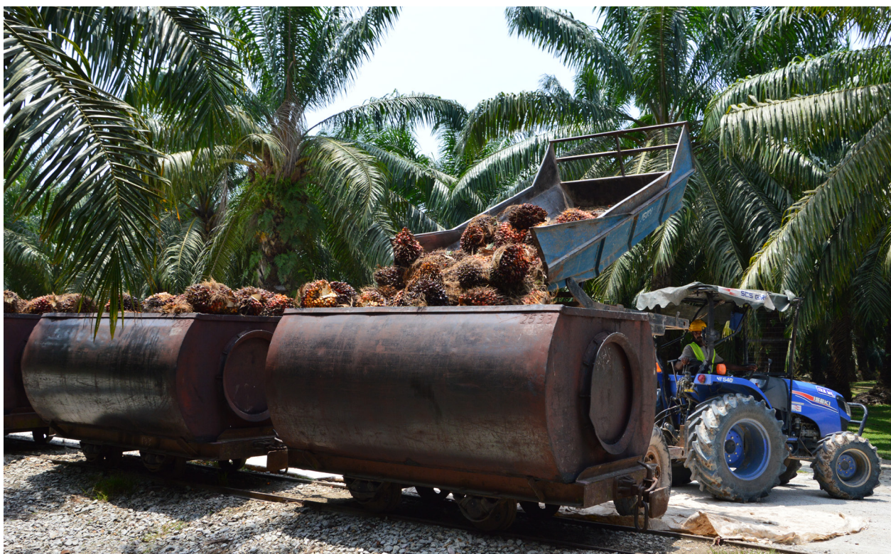
Mechanical assisted crop evacuation with tractor scissor lift trailers which enable considerably higher productivity vis-à-vis wheel barrow.
