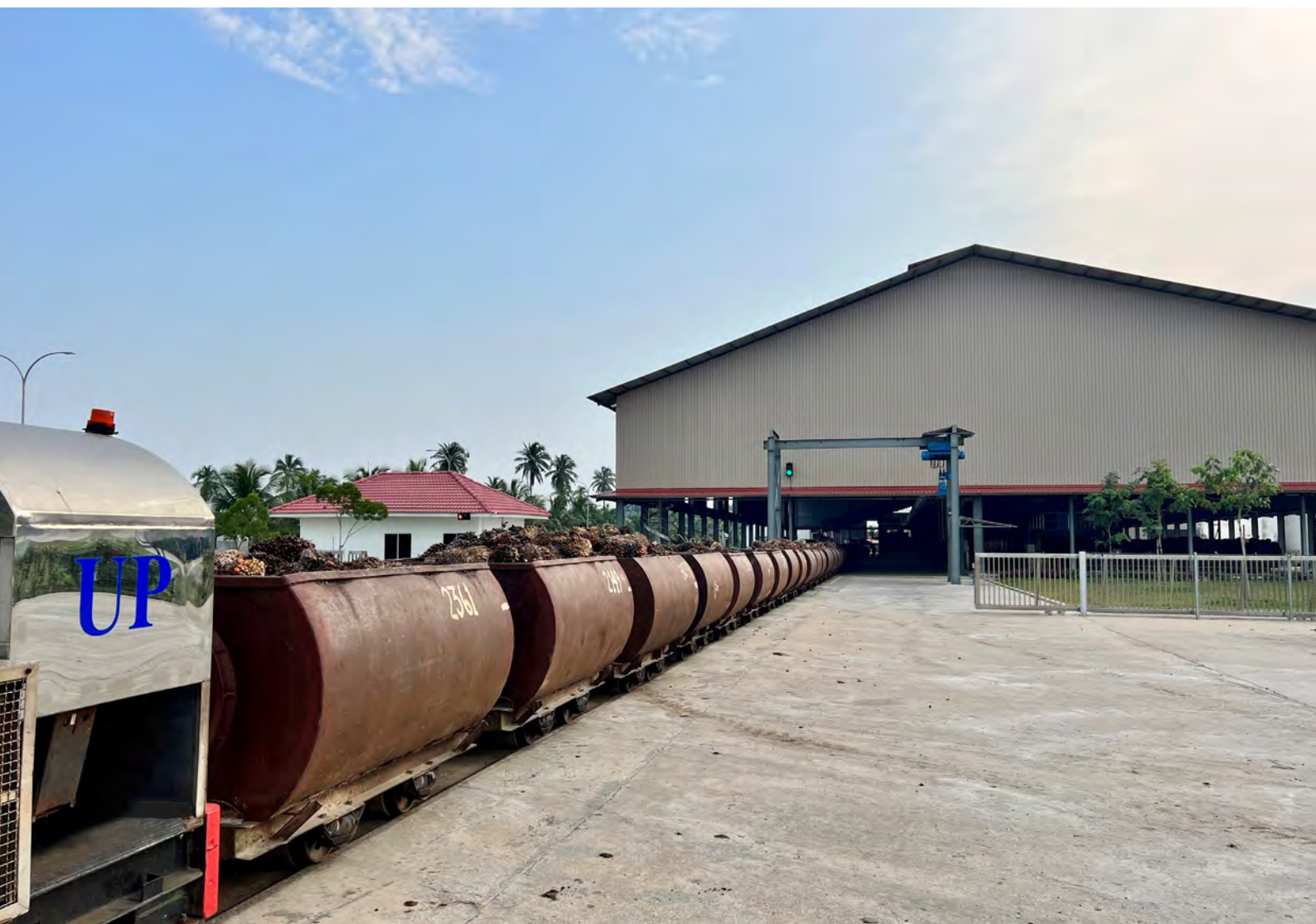
One of our locomotives bringing cages laden with freshly harvested fruit bunches to our recently upgraded palm oil mill on Jendarata Estate, where the fruits are cooked under pressure before further processing into high quality oil.
